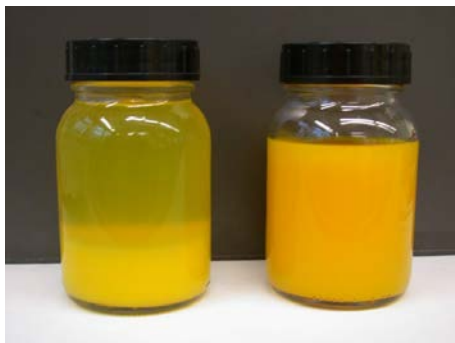
Figure 4 Before homogenisation – the filling agents settle on the bottom (left). Thorough stirring ensures a uniform distribution of the components (right).
