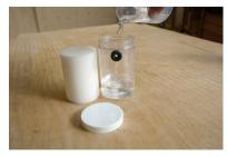
**Step 3:** Fill the climate control container with 150 ml of water. It is sufficient to check the water level every three months.
