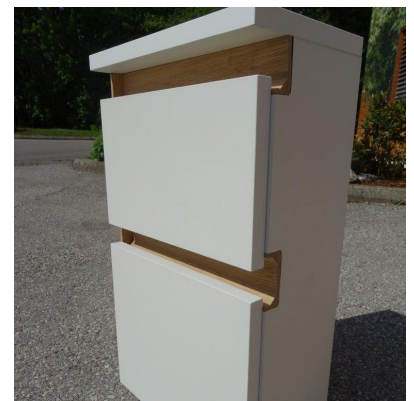
finished carcass with oak handles (L- and C-profile) and one-sided gap closure
