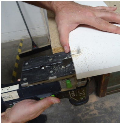
cutting a recess into the lateral part of the carcass
