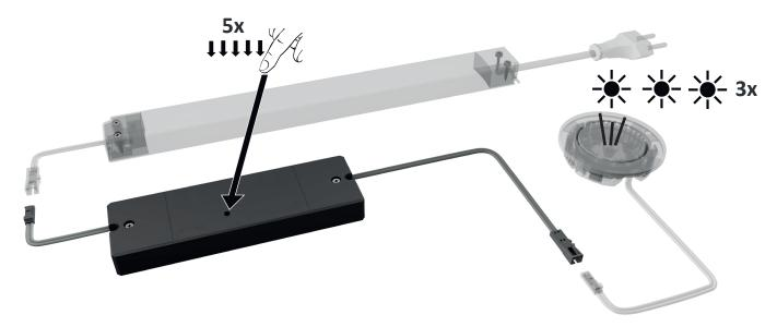
If the device has already been mounted in an inaccessible location, the functions can be carried out by disconnecting it from the mains (unplug and plug in) the same number of times in immediate succession.
