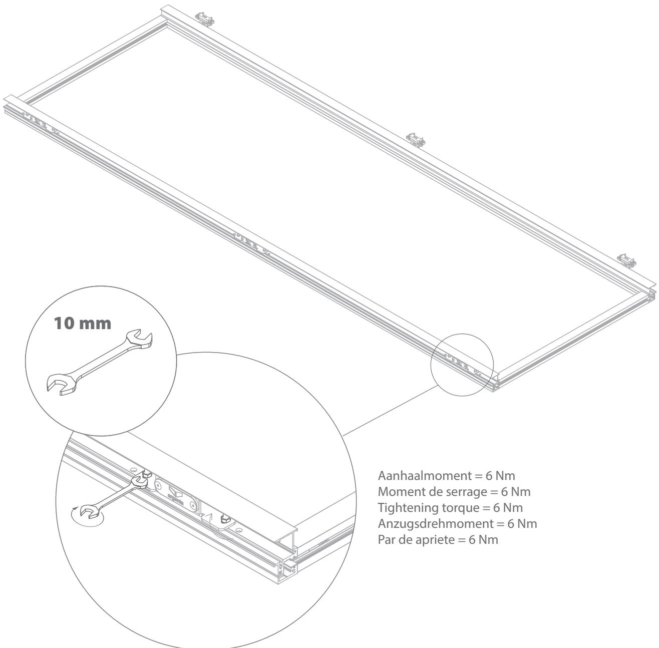
DEURMONTAGE AAN KADER / MONTAGE DE LA PORTE SUR LE CADRE / INSTALLING THE DOOR ON THE FRAME / TÜRMONTAGE AM RAHMEN / MONTAJE DE LA PUERTA EN EL MARCO
